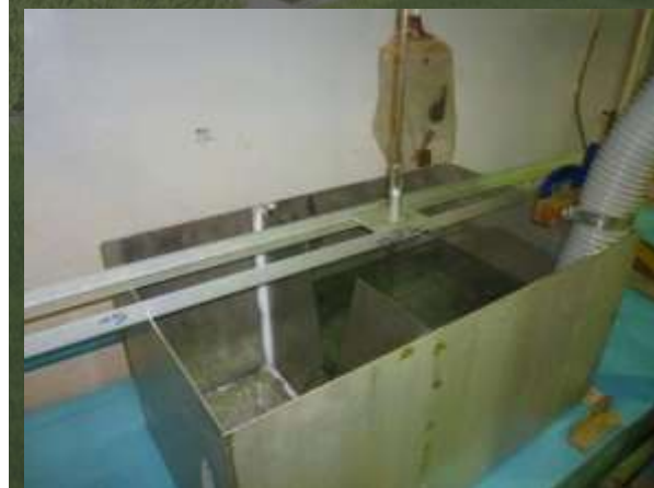
V-notch calibration setup in Hydraulics Laboratory
