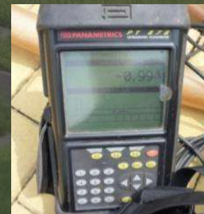
Runoff experiment setup (left) and ultrasonic flow meter (right)
